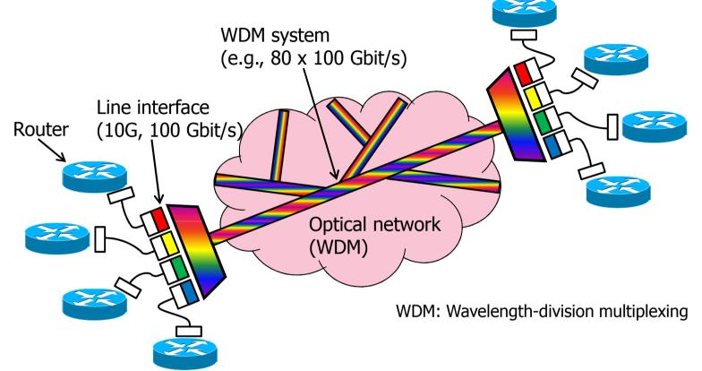
Key Technology #1: WDM = Solution to reach multiterabit/s capacity Key Technology #2: OTN = Solution to transport IP over DWDM
